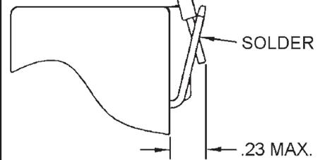
CONNECT THE TERMINALS OF LEADWIRE ASSEMBLIES 47 AND 48 TO THE TABS ON THE BOTTOM OF THE SWITCH AND SOLDER.
