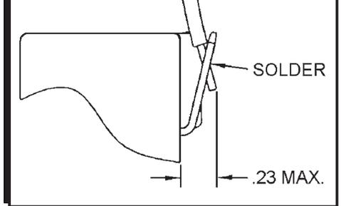
CONNECT THE TERMINALS OF LEADWIRE ASSEMBLIES 47 AND 48 TO THE TABS ON THE BOTTOM OF THE SWITCH AND SOLDER.
