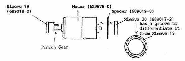
Type 2 Motor can be used with Type 3 Gear by replacing Pinion Gear on Motor (Part #221920-7) to Type 3 Motor's Pinion Gear (Part #221882-9).
